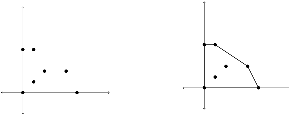
(a) Plot (i, j) for every nonzero monomial x^i y^j . (b) Draw the convex hull. The inside points are excluded from the final polygon.
