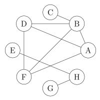
The vertices A, B, D, F form a clique of size 4 on G, and we also call this a *fully connected* subgraph of G. Similarly, the vertices C, E, G form an anticlique on G.
