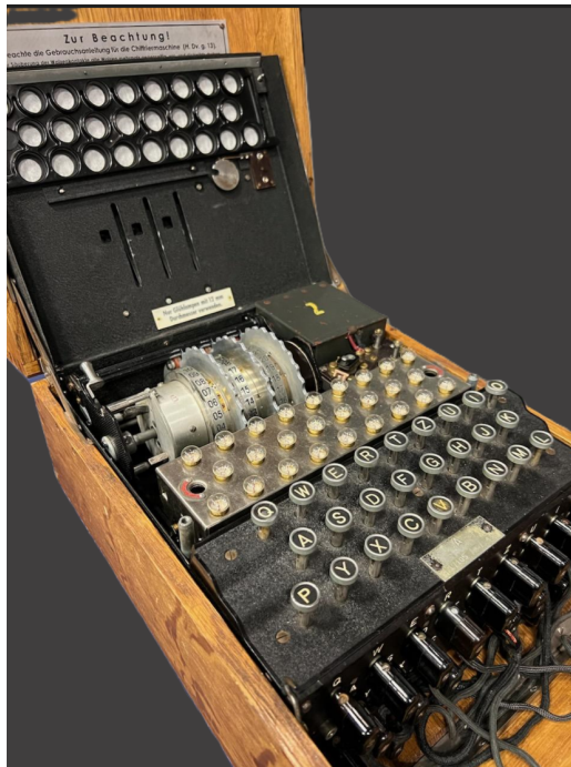
Figure 1: A commercial Enigma which has been re-wired to allow for modern battery use. Note that the cover over the lampboard and rotors has been lifted.
