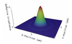
This is the Point Spread Function (PSF), which describes the system's ability to capture a point source. From here, take a vertical slice that runs through the center, and plot the intensity as you move across the slice. Now take the radial average for all such possible slices, or in other words, for each radius from the center take an average of the intensity values as you rotate about the center. The resulting graph is the Line Spread Function (LSF)
