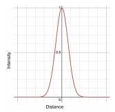
Taking the Fourier Transform of this converts from the space domain, with distance against intensity, to the frequency domain, with signals per distance as the input. This is our Modulation Transfer Function (MTF), which describes how clearly each spatial frequency is captured by the imaging system and the decrease in clarity as image complexity increases.
