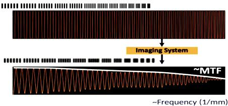
Here each peak captures a 'signal' and each quarter-period between a peak and a trough captures an 'edge response'. The amplitude of the curve across spatial frequencies captures this intuition of quantifying blur as signals get closer together, progressing towards indistinguishable grey with high frequency.
